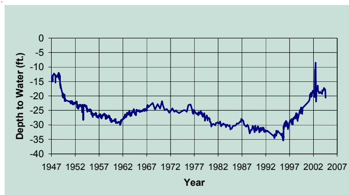
FIGURE 2. A general decline in water levels changed after 1994 when Moorhead began taking more water from the Red River of the North (data from ground-water-level monitoring well 14001 in the Buffalo aquifer).
