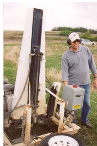
FIGURE 2. DNR hydrologists may use seismic equipment to assist with geologic mapping of potential aquifers. The seismic data complements existing well data.
