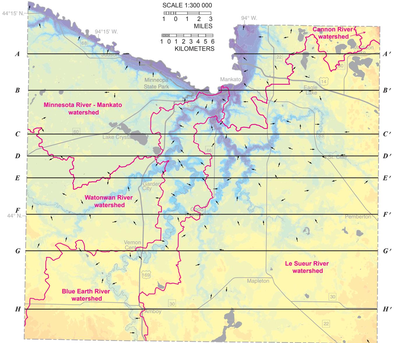
**Water-table elevation (feet above mean sea level)**
