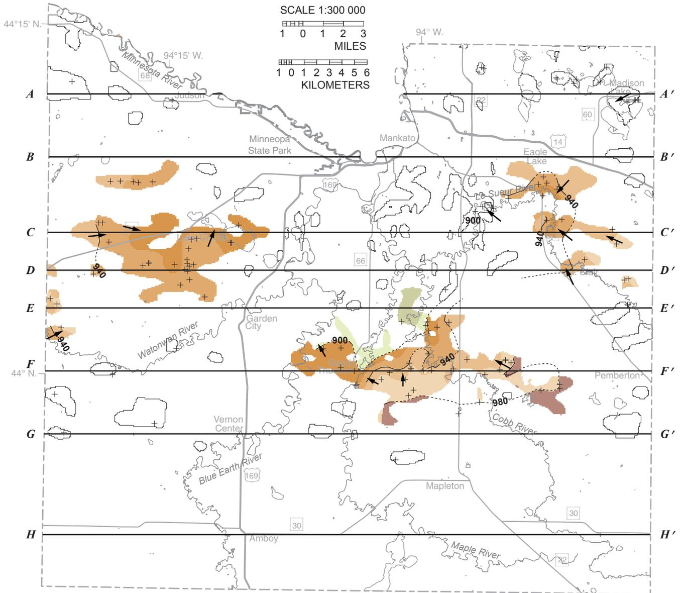
**Potentiometric surface elevation of aquifers**
