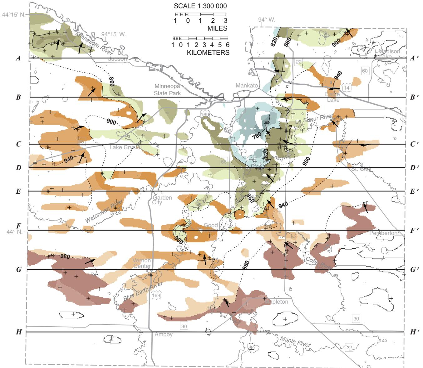
**Potentiometric surface elevation of aquifers**
