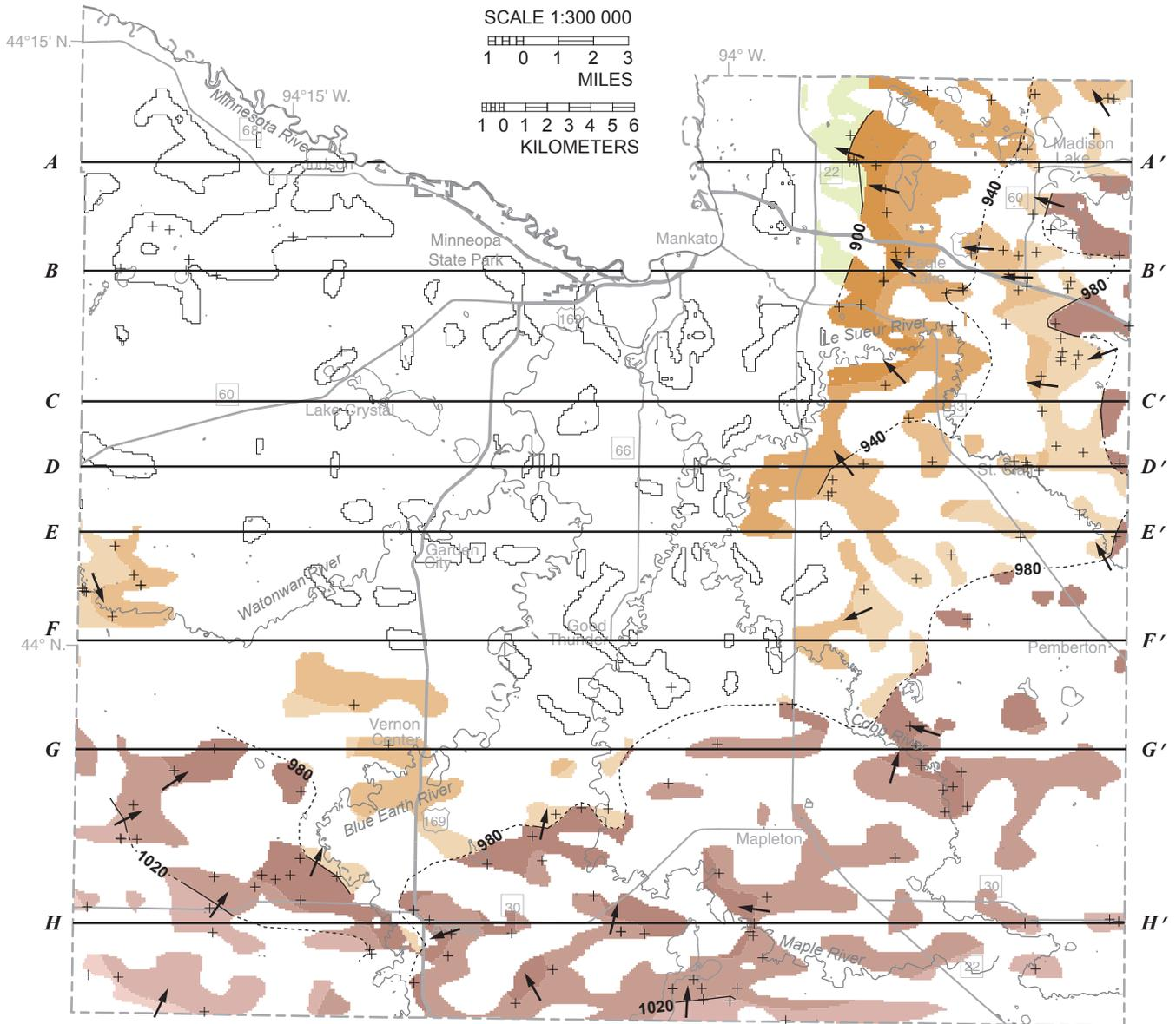
**Potentiometric surface elevation of aquifers**
