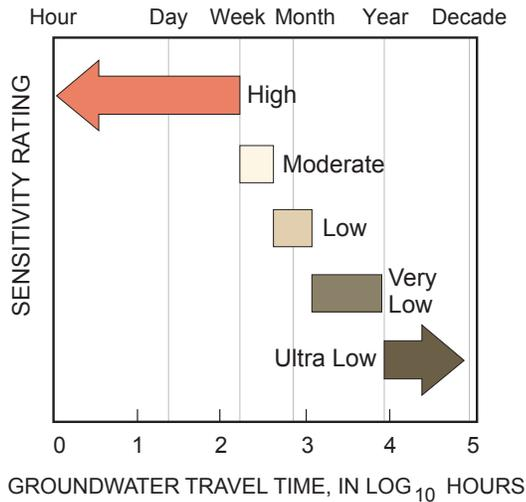
**Figure 20. Geologic sensitivity rating for the near-surface materials**
