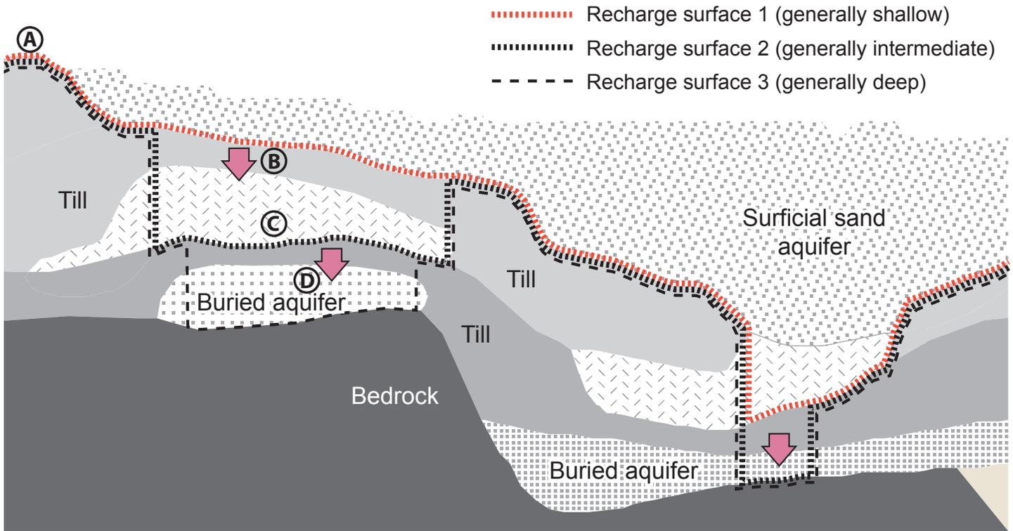
**Figure 23. Generalized cross section showing recharge surfaces for sensitivity evaluations of buried aquifers and bedrock surface**
