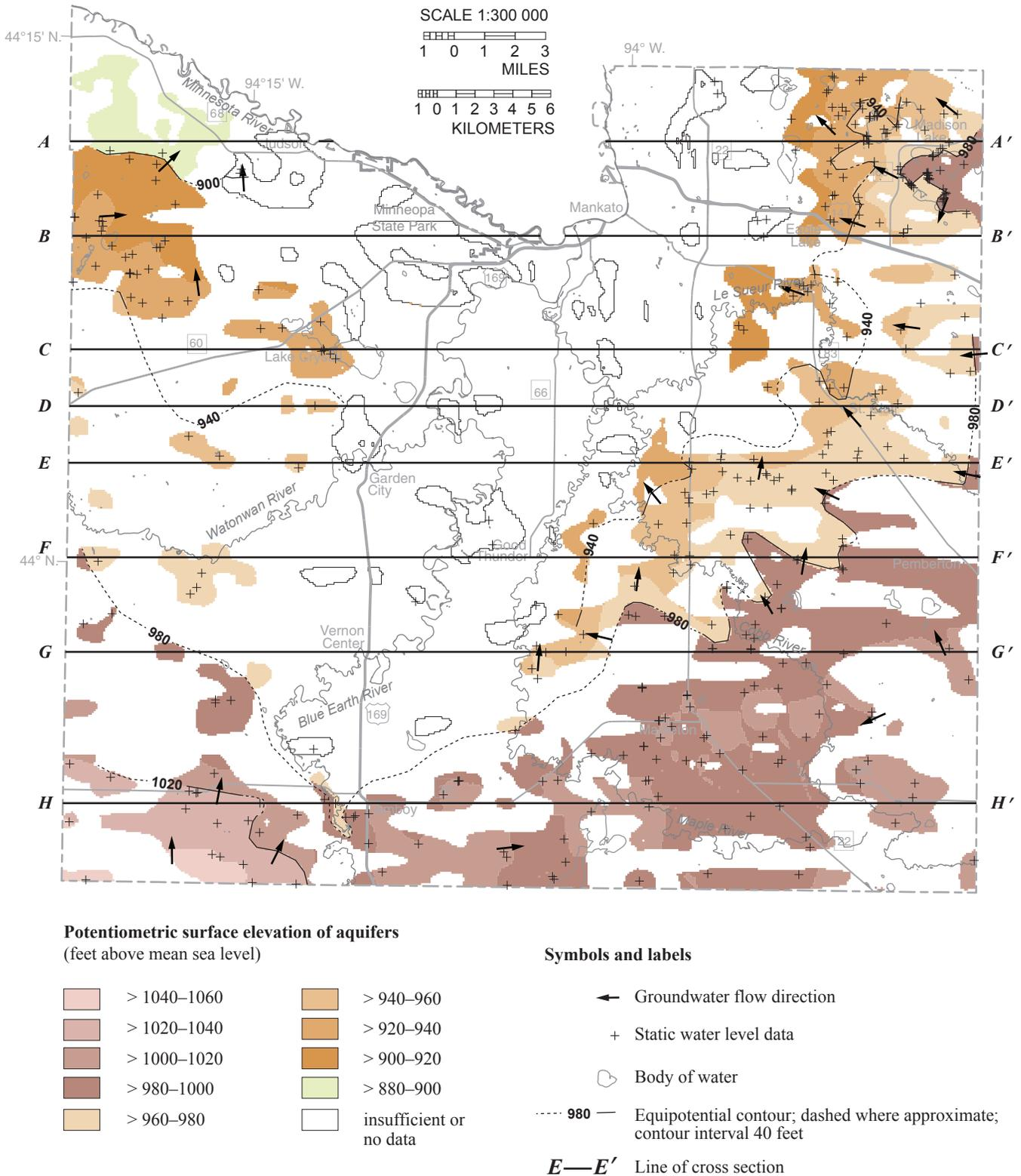
**Figure 9. Potentiometric surface of the st aquifer**
