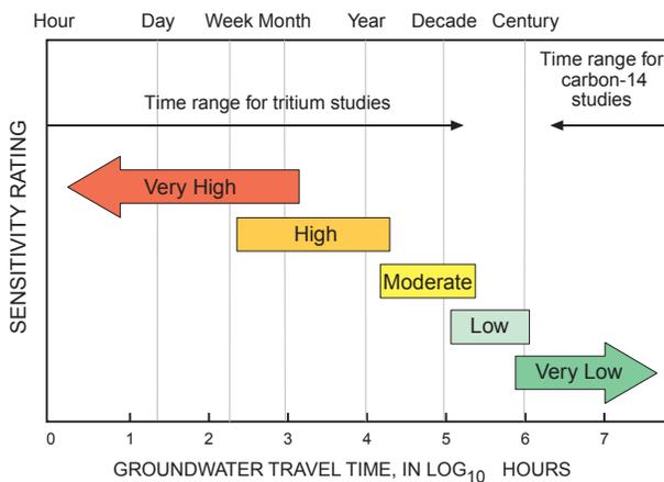
**Figure 21. Geologic sensitivity rating for the buried sand aquifers and the bedrock aquifers**
