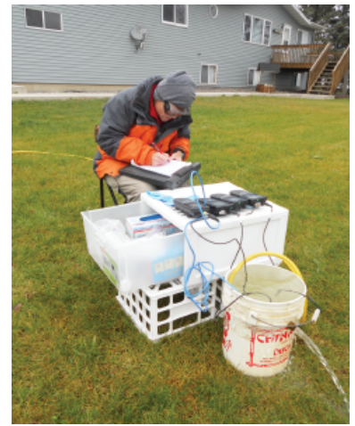
DNR hydrologist records data collected onsite from a residential well using various meters.
