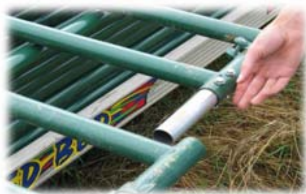
Figure 13. EMT conduit used to assemble gates.
