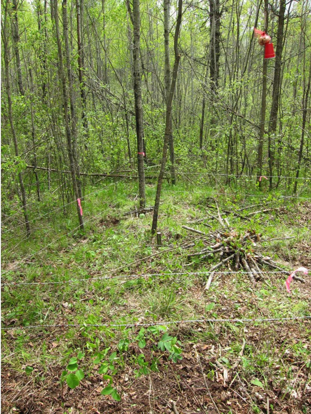
Figure 2. Set-up of barbed wire hair snare, showing 2 strands of barbed wire, central pile of bait and scent, and suspended bait and scent cup.
