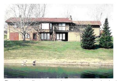
These pictures illustrate vegetation management in a shoreland area that is bad (above) and good (below). In the top picture, turf and the absence of a vegetative buffer allow runoff to easily follow the slope to the water. That runoff may cause erosion or carry contaminants or nutrients to the surface water. In contrast, the picture below shows a heavy vegetative buffer protecting the water. Additionally, the presence of emergent vegetation reduces the impacts of wave action on the shoreline.
