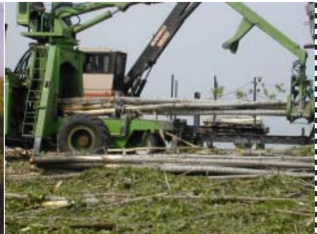
Hahn Harvester processing poplar trees. This machine made the tree limbing feasible.
