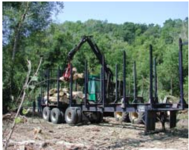
Loading boxelder directly onto the forwarder
