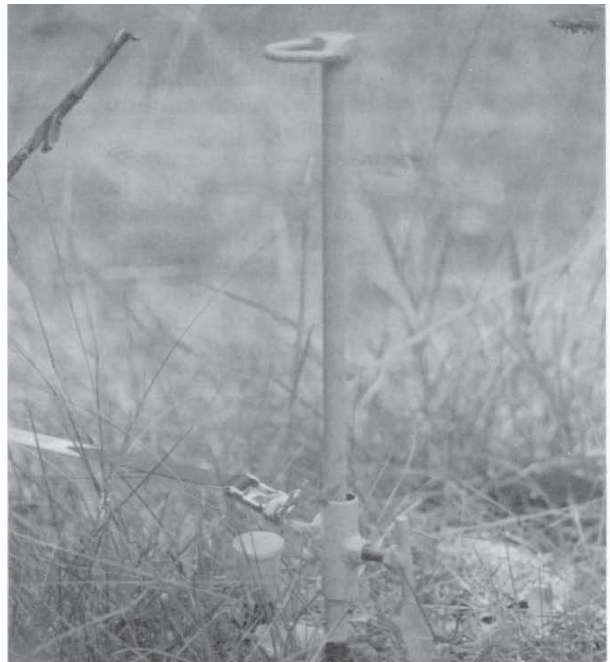
Figure 15. Rebar monument at cross-section (capped rebar on left, next to silver stake).
