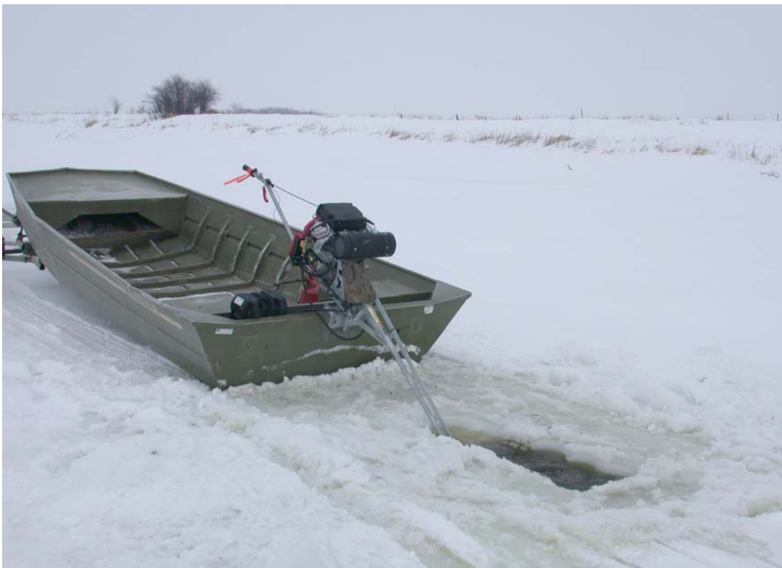
Appendix 24. Outboard mud motor in operation during a reverse aeration treatment of Danielson Pond (Big Stone Co., Minnesota), 5 Feb 2004.
