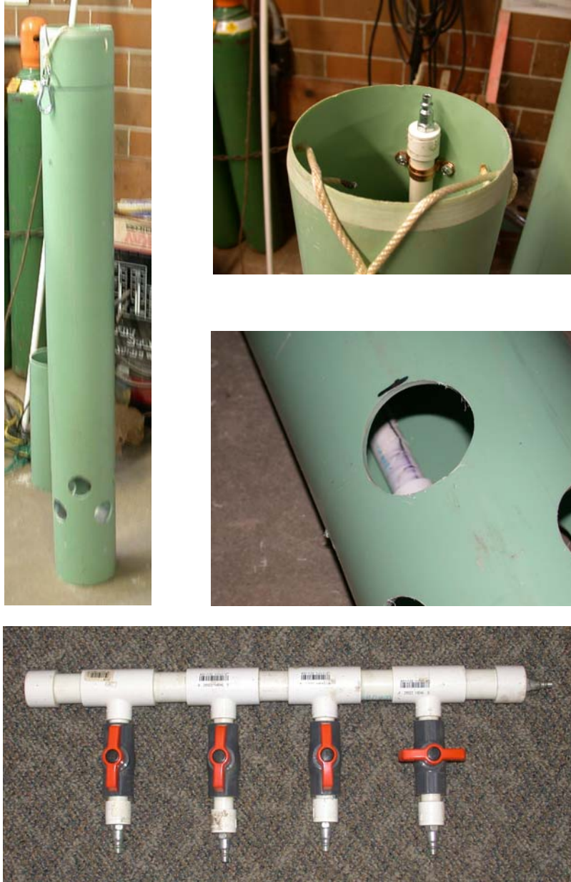
Appendix 23. Airlift tube and air line manifold used for treating ponds > 15 ft deep. The manifold was constructed from standard hardware; it allowed running up to 4 airlift tubes from a single air compressor. The airlift tube was made from 6 in diameter by 4.5 ft long SDR sewer pipe. About 6 in of ready-mix concrete was poured in the bottom and held in place with a horizontal piece of steel rod stuck through two holes in the pipe before adding the concrete. There were eight 2.25 in diameter holes in two rows just above the top of the concrete. Inside the main tube was an air diffuser made from ½ in diameter PVC pipe, capped on both ends, with a standard air-line fitting screwed into the top, and several air escape slits cut near the bottom with a hacksaw. The diffuser assembly was attached to the inside of the sewer pipe near the top and bottom with standard hardware, and was flush with the top of the pipe. The bottom of the diffuser extended down to just above the holes at the bottom of the pipe. A rope was attached to the top of the pipe for raising and lowering the tube without pulling on the air line.
