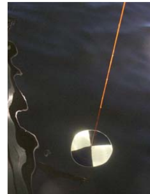
Figure 4. Measuring water clarity with a Secchi Disc
