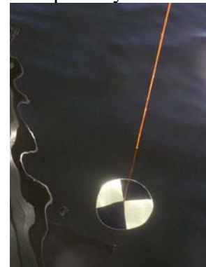
Figure 4. Measuring Secchi Disc transparency
