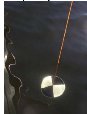
Figure 3. Measuring Secchi Disc transparency
