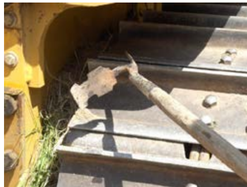
Right photo: Tool for scraping out soil and plants
