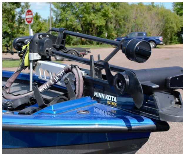
A trolling motor attached to the bow of a watercraft.
