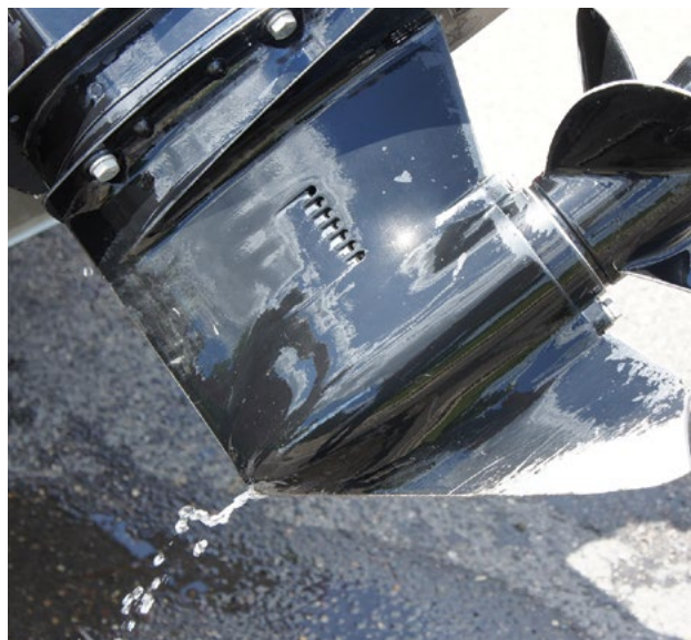
Water draining from a lower unit
