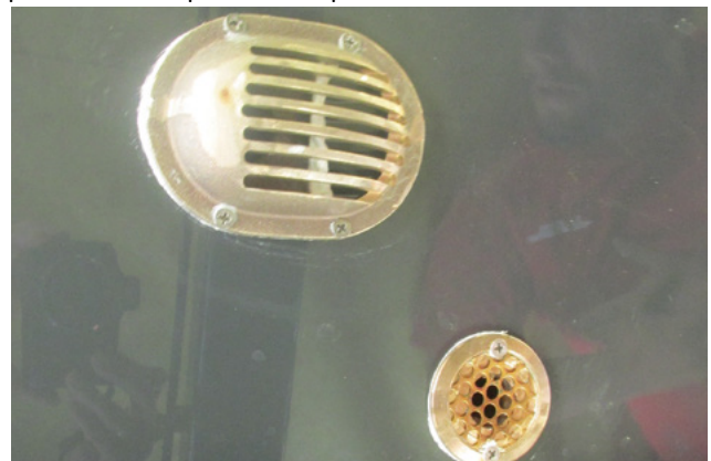
Inboard engine intake (large oval) and ballast tank intake (small round)
