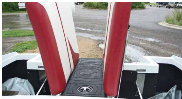
Location of soft ballast tanks in a wakesport boat.
