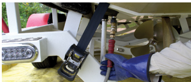
Fake-a-lake attachment used to fill a ballast tank from the bottom thru-hull fitting.
