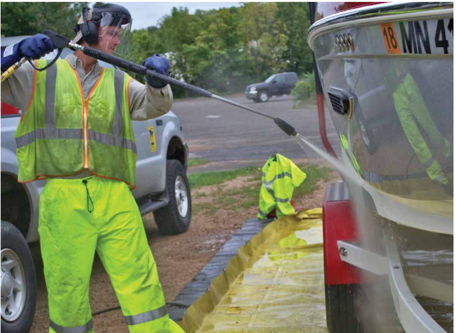
Hot water, high pressure spray of a watercraft hull.
