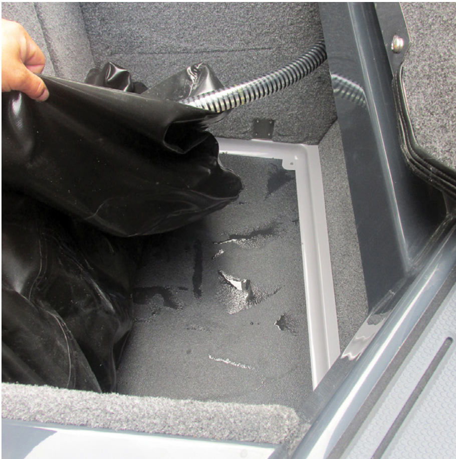
Ballast tanks can be installed underneath floors, and oftentimes a watercraft can have hard and soft tanks in the same area.
