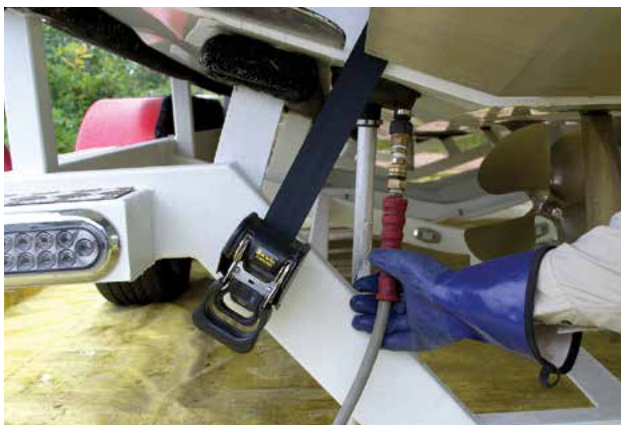
Fake-a-lake attachment used to fill a ballast tank from the bottom through hull fitting.
