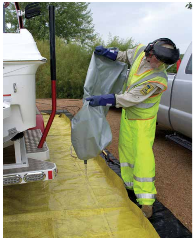
Inspector removes a soft ballast tank.
