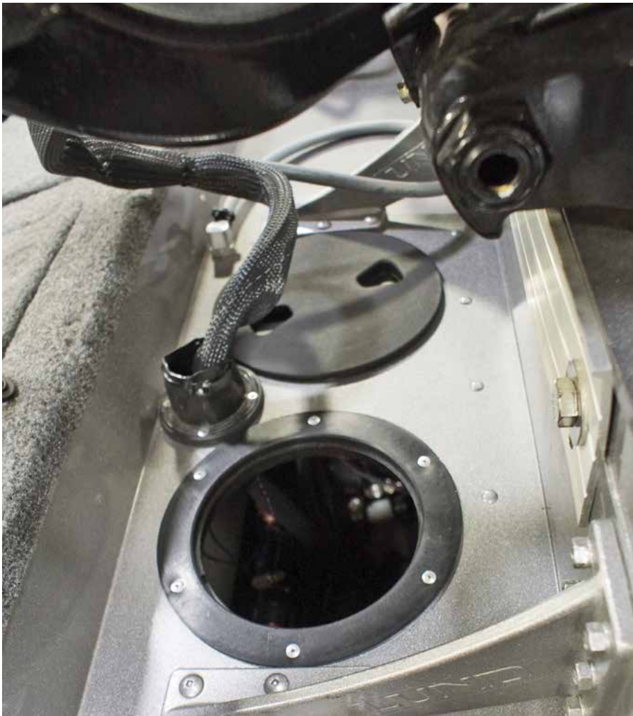
Bilge areas are often tight spaces. An inspector may see residual water but be unable to sponge it out.
