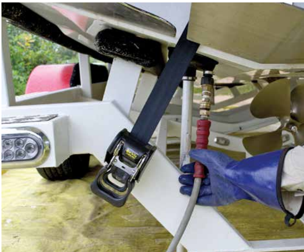
Fake-a-Lake is positioned over the water intake.
