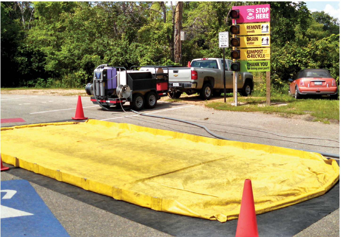
Observe the traffic flow of the access when setting up the decontamination area; consider safety of the inspector and the public first.
