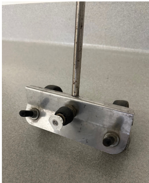
An undercarriage sprayer can be attached to a cradle with one or more wheels to increase mobility and stability.
