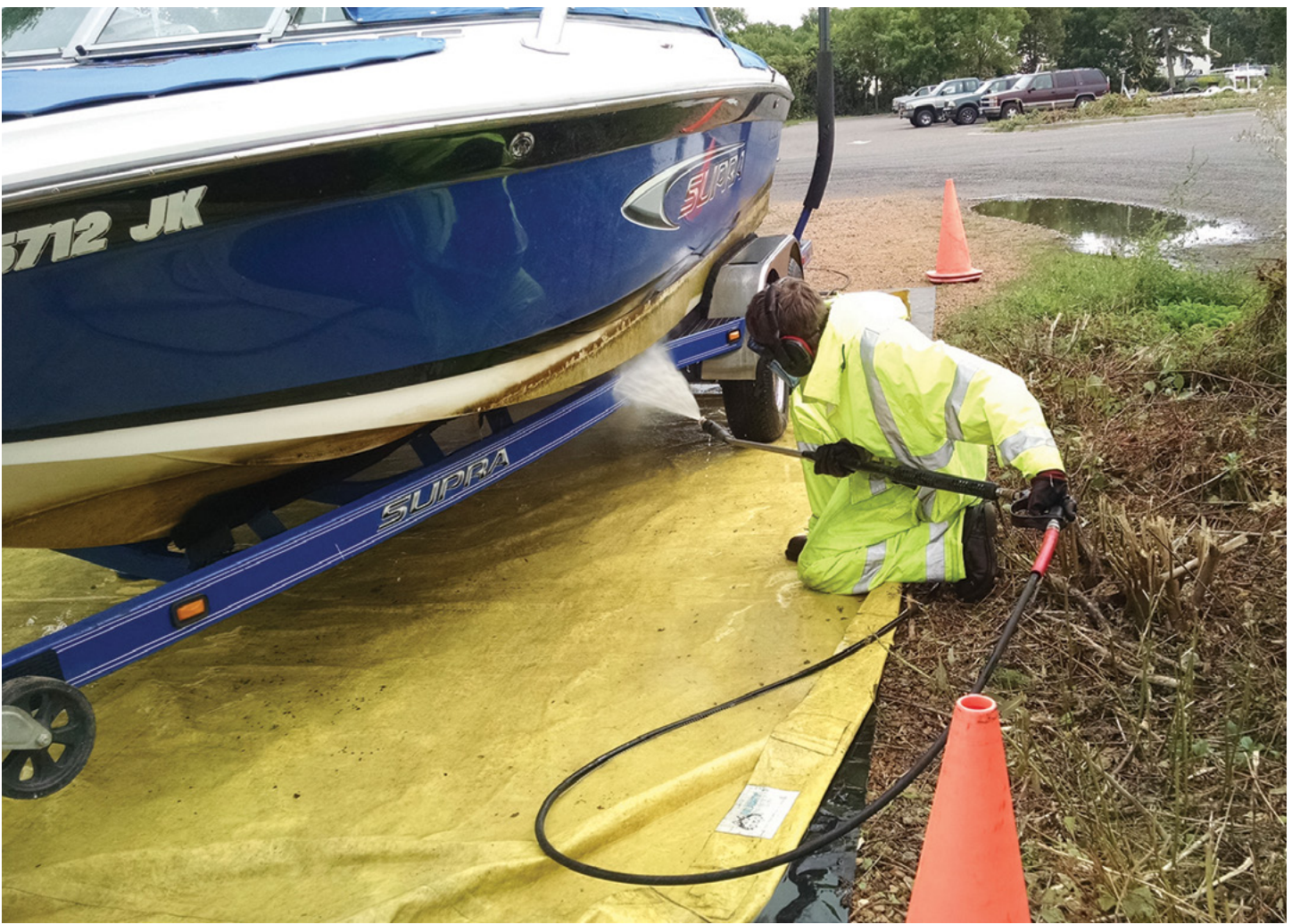
An inspector crouches down to use high-pressure spray on the underside of a hull in order to complete a full decontamination.
