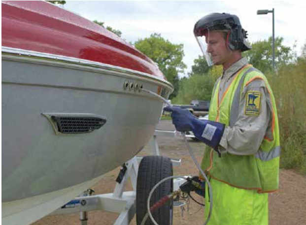
Inspector uses ballast tank diffuser hose to flush 120°F water into a ballast tank. The water is held in the tank for at least 5 minutes before being pumped out.
