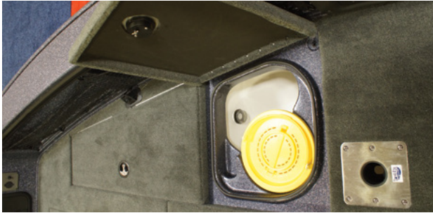
Check all water-holding compartments, like this baitwell, to ensure they have fully drained.
