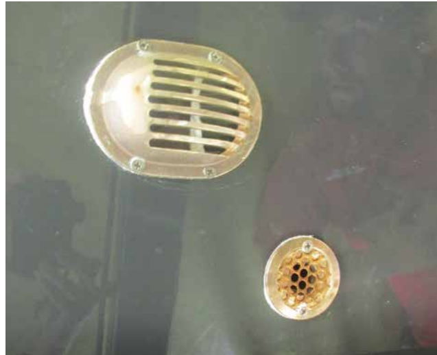
Inboard engine intake (large oval) and ballast tank intake (small round)
