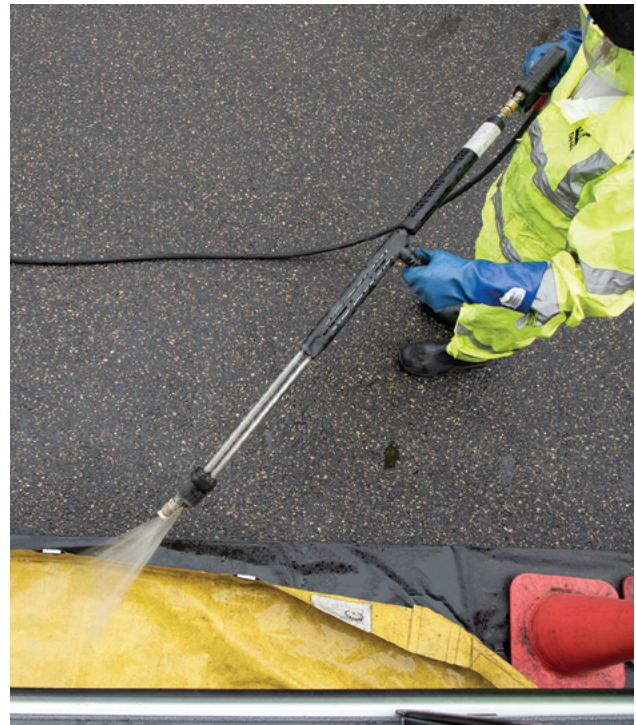
Inspector uses high-pressure spray at a 45° angle from the hull.
