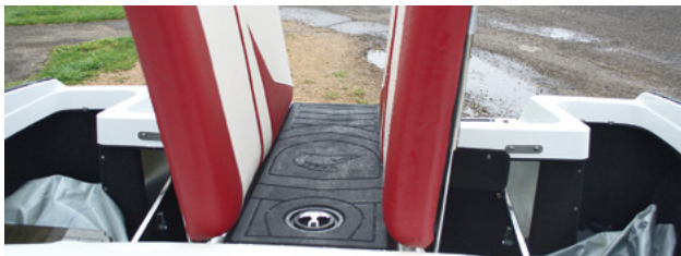
Location of soft ballast tanks in a wakesport boat.
