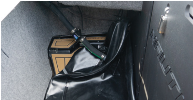
Work with the watercraft operator to ensure all ballast areas are free of residual water.
