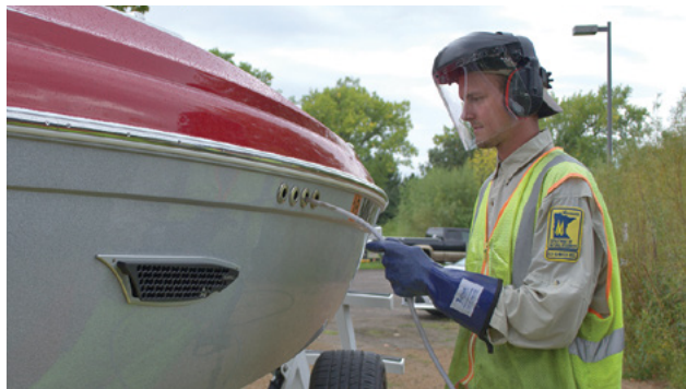
Inspector uses ballast tank hose to flush 120°F water into a ballast tank. The water is held in the tank for at least 5 minutes before being pumped out.
