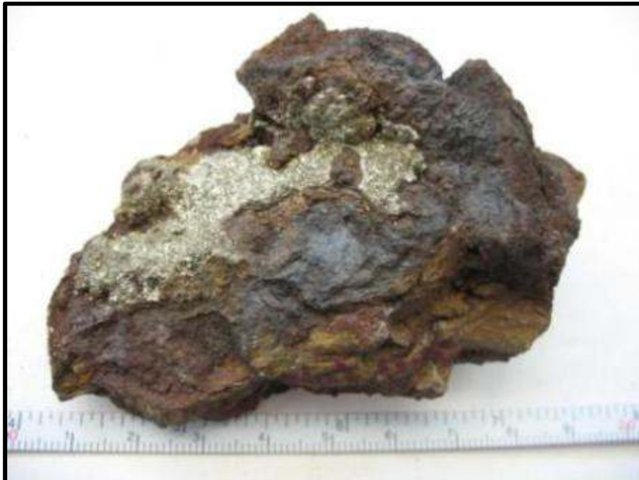
Figure 40: Natural ore containing fine grained, euhedral pyrite aggregates, Fayal Mine.
