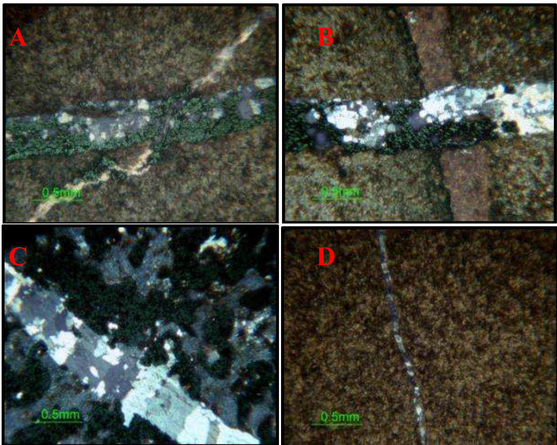
Figure 39: Secondary sulfide minerals located in veins; A. Calcite vein cross cutting quartz vein, both containing pyrite (MGS-5-13); B. quartz and calcite vein containing pyrite (MGS-5-13); C, D. Quartz only vein with no sulfides present (MGS-5-6, MGS-5-13), all slides seen under transmitted and reflected light microscopy.
