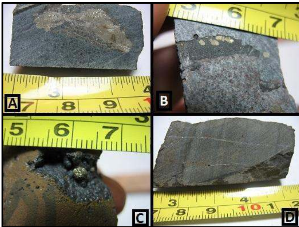
Figure 33: Different types of sulfide occurrences. A. anhedral mass (MGS-5-21); B. euhedral cubes (MGS-7-17); C. framboidal (MGS-8-16); D. vein (MGS-5-15).
