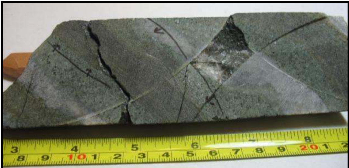
Figure 35: Core sample B1-305-16 showing layered concentrations of pyrrhotite and magnetite in a metamorphosed section of the Biwabik Iron Formation.
