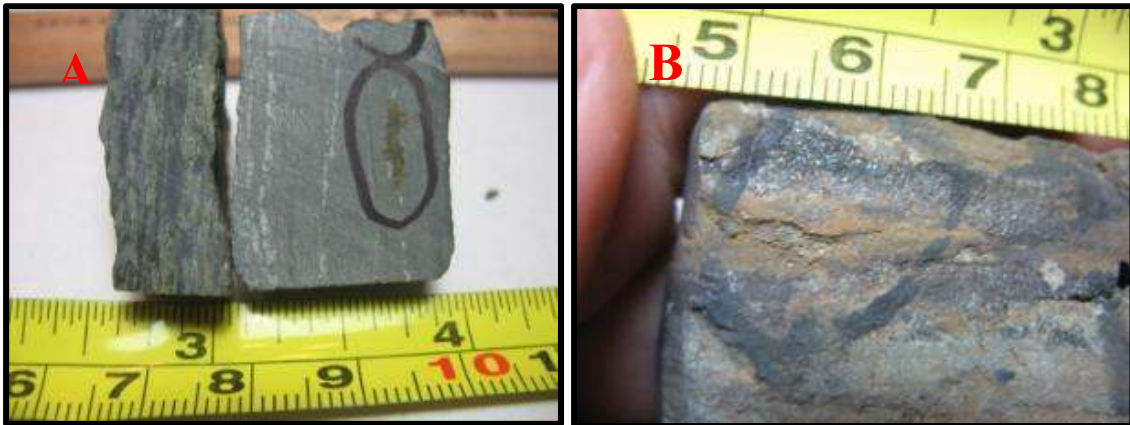
Figure 36: Massive, strata-bound, secondary sulfide masses/aggregates. A. Anhedral sulfide mass located in association with calcite in sample MGS-2-2 B. sulfide aggregation in leached layers in sample MGS-8-4.
