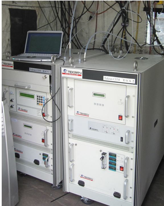
Photograph 3. Tekran Mercury Conversion Module and CEM
