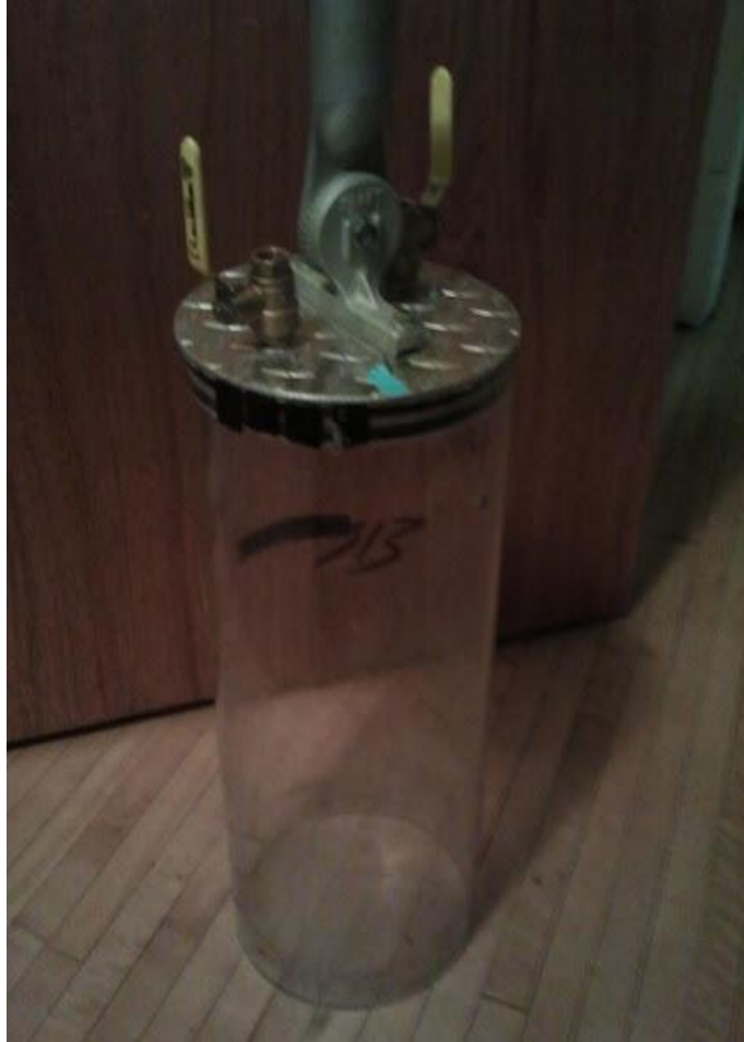
Figure 3. Sediment Core tube attached to sediment corer and drive rod. Ball valves displayed in an open position, which was used when driving core tube into sediment and closed 90° when core had reached its desired depth.
