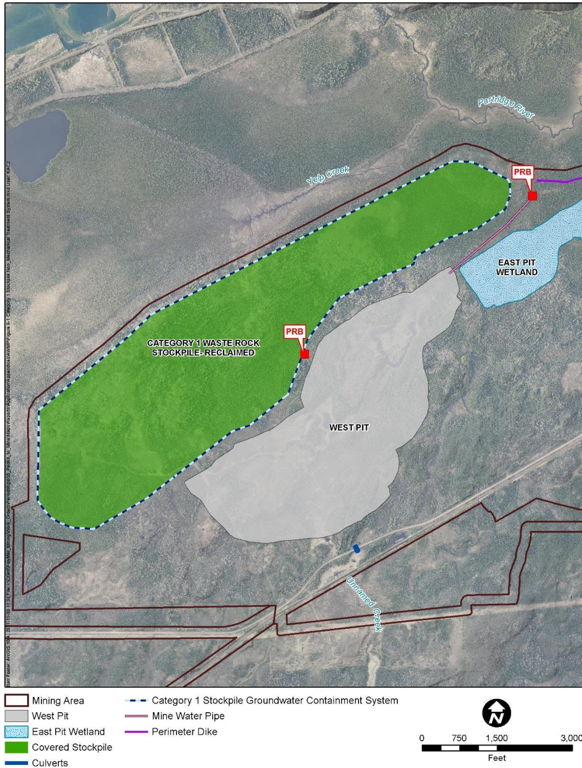
Figure 6-1 Conceptual Plan View: Category 1 Stockpile Non-Mechanical Treatment System
