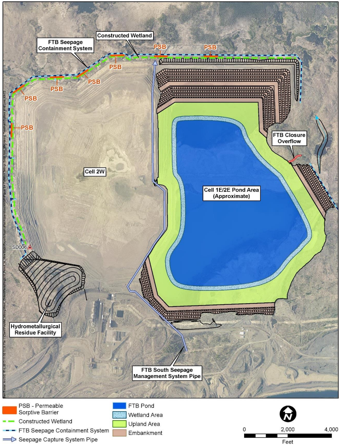
Figure 6-4 Conceptual Plan View: FTB Non-Mechanical Treatment System
