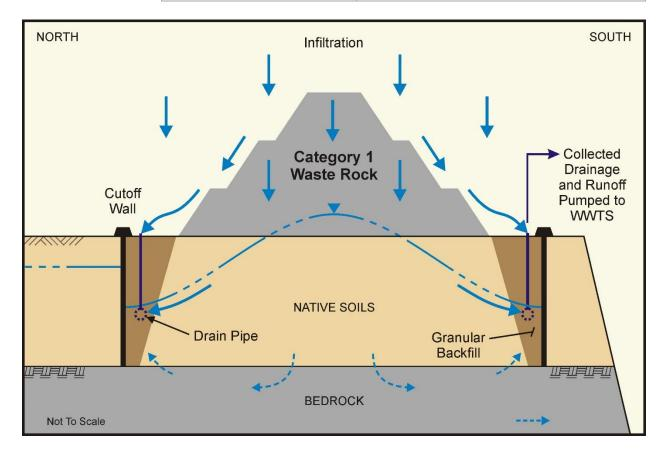
Figure 2-2 Conceptual Representation of Category 1 Stockpile Groundwater Containment System – Operating Conditions Cross-Section
