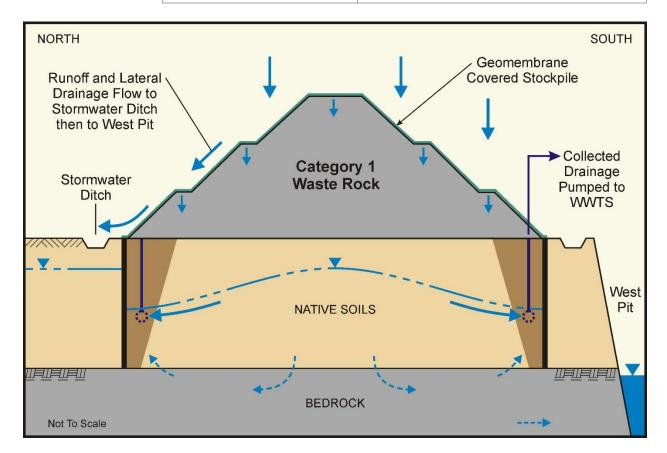
Figure 7-1 Conceptual Representation of Category 1 Stockpile Groundwater Containment System – Reclamation and Long-Term Conditions Cross-Section
