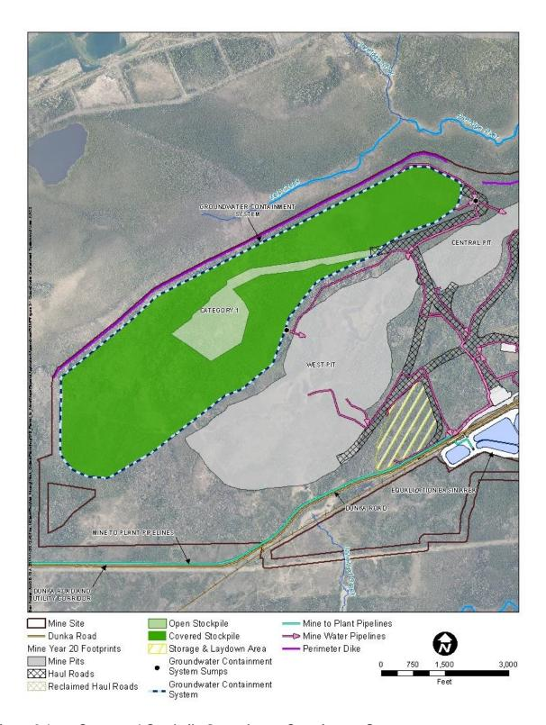
Figure 2-1 Category 1 Stockpile Groundwater Containment System
