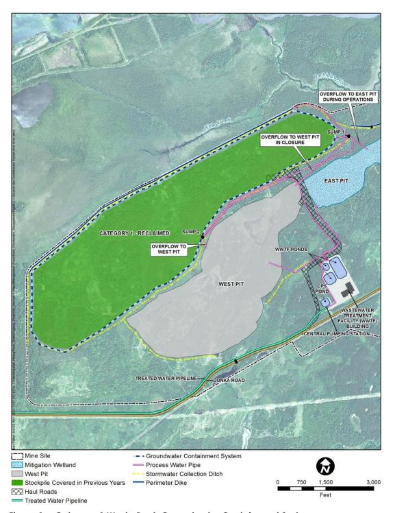
Figure 1 Category 1 Waste Rock Groundwater Containment System
