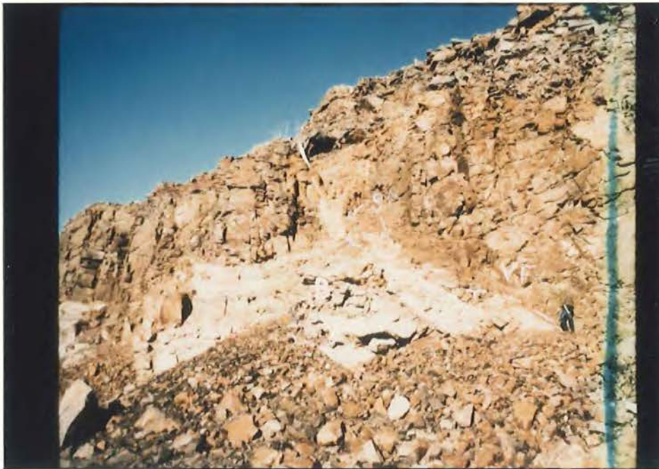
Figure III-1: A: Thrust fault in the south pit of Erie Mine Area #8. Granite is intruded along the fault plane in the upper part of the photo. View to the east. gr = granite; VF = Virginia Formation; B = diabase sill; b,c = layers of banded iron formation. B: Close-up of III-1A.
