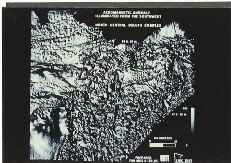
Figure 8. Total magnetic intensity anomaly over the central Duluth Complex. Shaded relief format illuminated from the southwest at 45° inclination.
