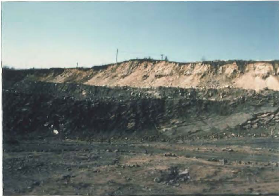
Figure II-1: Folding in the Lower Cherty Member of the Biwabik Iron Formation along the Denora Fault at the west end of the Erie Mining Company Area #1. View is looking southwest.
