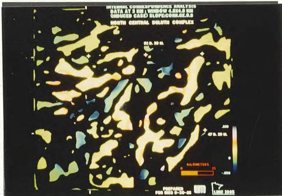
Figure 17. Poisson analysis, dJ/dp estimates based on reduction to pole assuming direction of induced magnetization (dec/inc = 5^{\circ}/75^{\circ} down). Areas where dJ/dp estimates are associated with low correlation coefficient values (smaller than \pm 0.80 ) are black.
