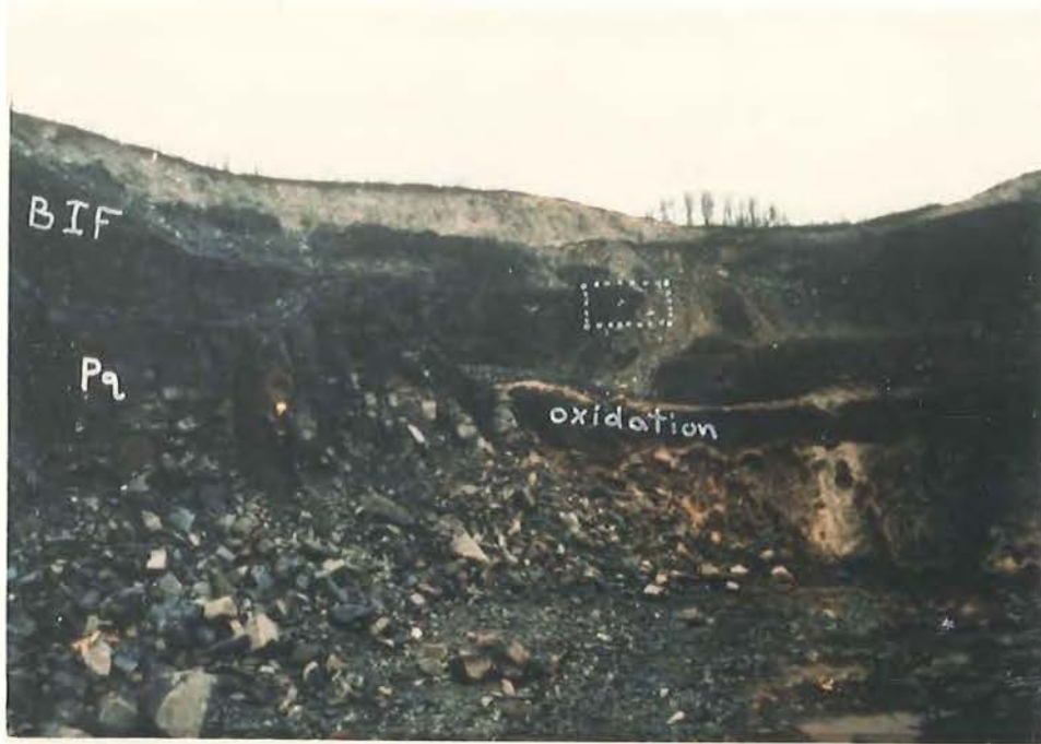
Figure II-2: Oxidation along the Denora Fault at the northwest end of the Denora Mine. The figure in the left-central portion of the photo is standing next to a bench face of Pokegama Quartzite (Pq). The dotted area outlines the area shown in Figure 3A. View here is to the northwest.
