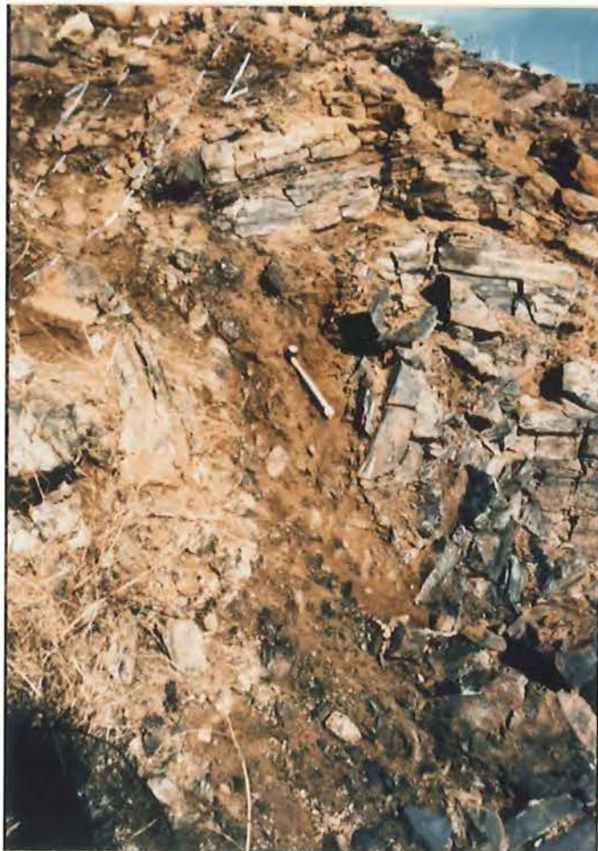
Figure II-11: A: Reverse fault (B-6) in Erie Mine Area #9S. The fault zone is shown dashed where exposed, dotted where covered. Note folding on downthrown side. View to northeast. B: Close-up of II-11A.
