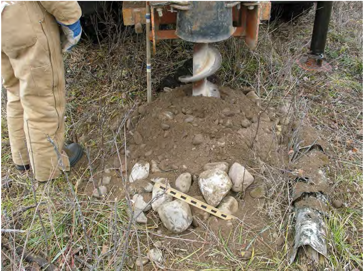
The above photograph shows the texture of the sand and gravel excavated at test hole 9 at the Industrial Township Site. The black bars on the scale are one inch long. The photo was taken October 23, 2006.
