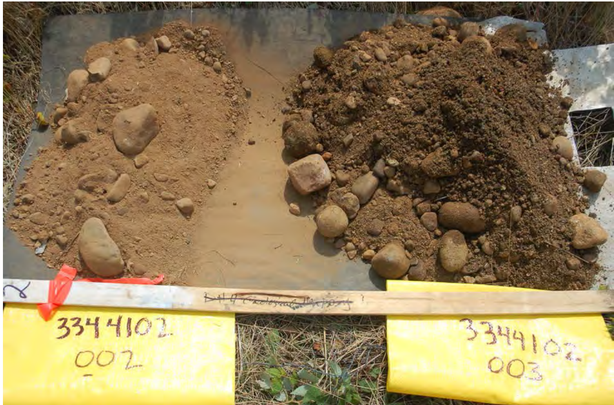
Figure 3. This photo shows the difference in the upper few feet of the gravel deposit compared to the deeper gravel in Test Hole 2. The light colored sample on the left is from the upper 2 feet of the hole and has a high percentage of fine sand. The gradation test indicates the sample on the left had 6.8% passing 200 sieve and the sample on the right had 2.0% passing 200 sieve.
