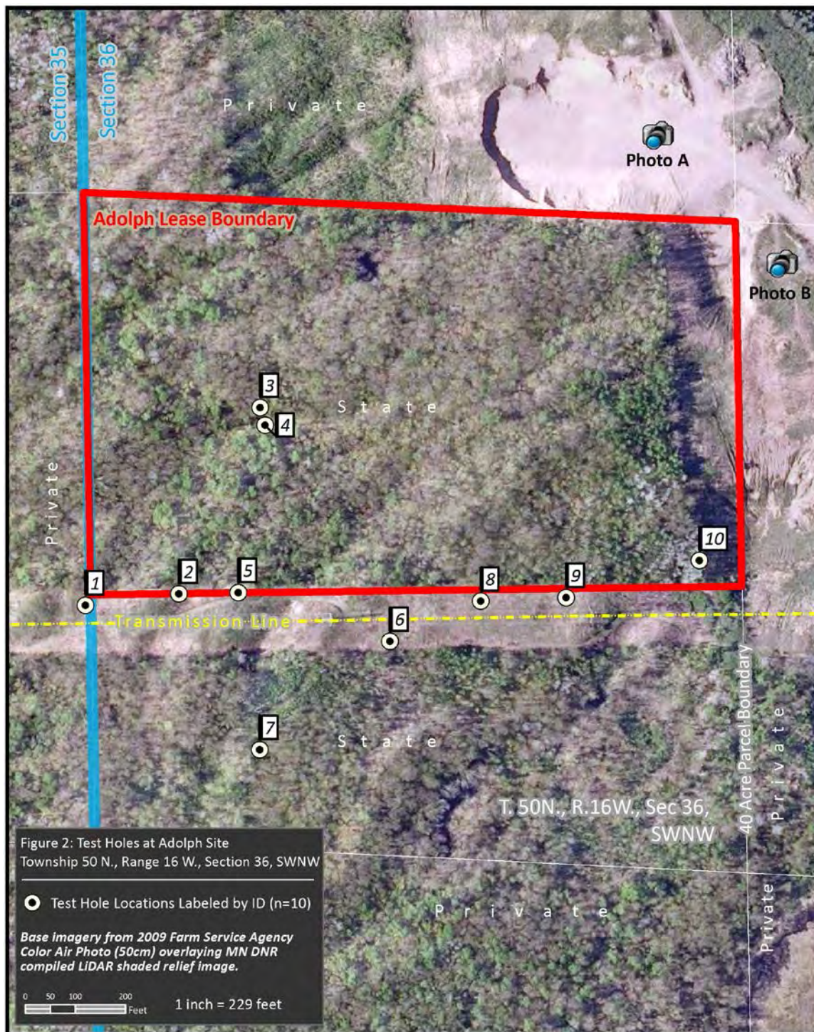
Figure 2. Ten test holes within and near the lease area are depicted as white circles filled with a black dot. The box adjacent to each circle includes the unique ID number for the test hole. Each hole was dug with an excavator to a depth of about 14 feet. The camera icons at the upper right portion of the figure show approximate locations from which a set of panoramic photos looking toward the state land were taken. These photos are found in Figures 3 and 4.
