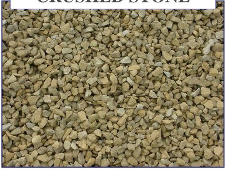
A product of mechanically breaking down bedrock like granites, quartzites, basalts and limestones.
