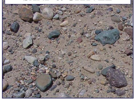
Naturally occurring sediment that has been sorted and deposited by flowing water.
