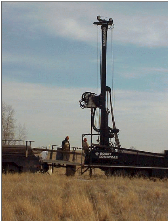
Figure 5A (Above): The rotosonic drill rig. 5B (Upper Right): Drill core being vibrated out of core barrel. 5C (Lower Right): Drill core getting labeled and boxed.
