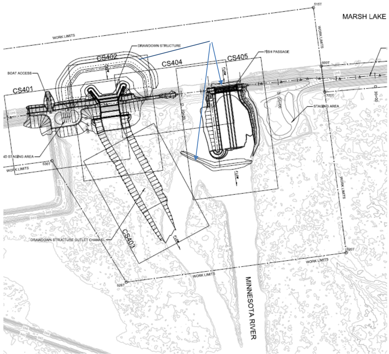
Figure 3. Locations of water control structure, fishway, west parking lot, and temporary coffer dams for Marsh Lake Dam.
