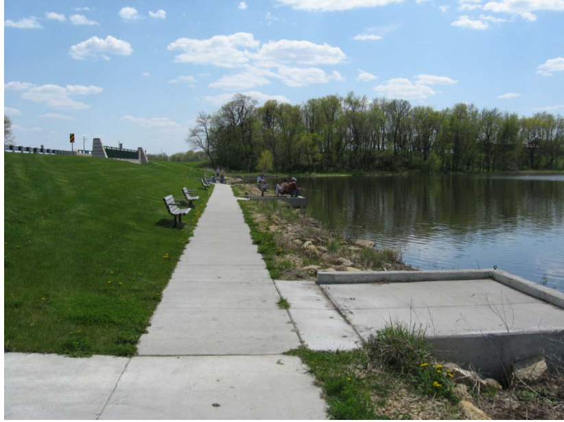
Figure 7-5. Example of an accessible shore fishing platform.
