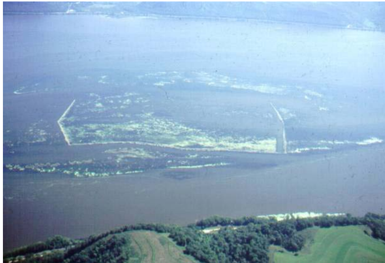
Figure 4-12. Constructed rock island sheltering aquatic vegetation. Pool 9, Mississippi River.
