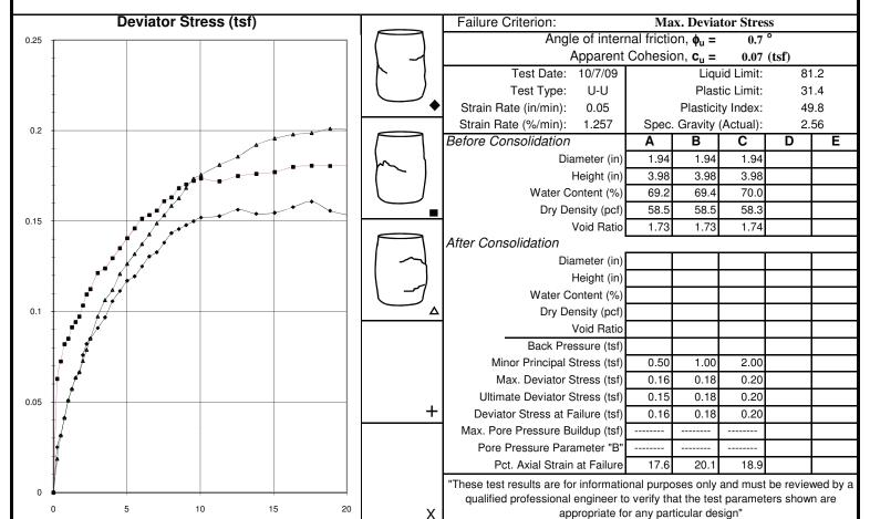
Remarks: Specimens trimmed to given sizes; Allowed to adjust under applied confining pressures for about 10 minutes.
