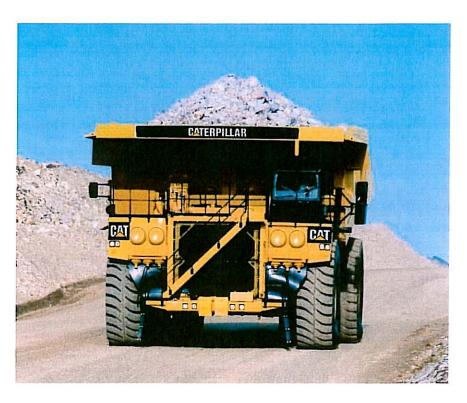
Integrated Braking System. The Cat oil-cooled braking system delivers reliable performance and control in the most extreme haul road conditions. The integrated system combines the service, secondary, parking brake and retarding functions in the same robust system for optimum braking efficiency.
