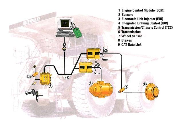
**Cat Data Link.** Electronically integrates machine computer systems to optimize overall power train performance, increase reliability and component life, and reduce operating costs.
