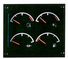
**Gauge Cluster.** Conveniently located gauge cluster maintains a constant display of vital machine functions, including:
