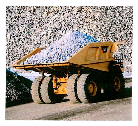
Mechanical Power Train. The Cat mechanical drive power train and power shift transmission provides unmatched operating efficiency and control on steep grades, in poor underfoot conditions, and on haul roads with high rolling resistance.
