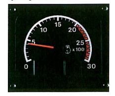
**Speedometer/Tachometer Module.**Monitors three systems: engine speed, ground speed and gear indicator.
