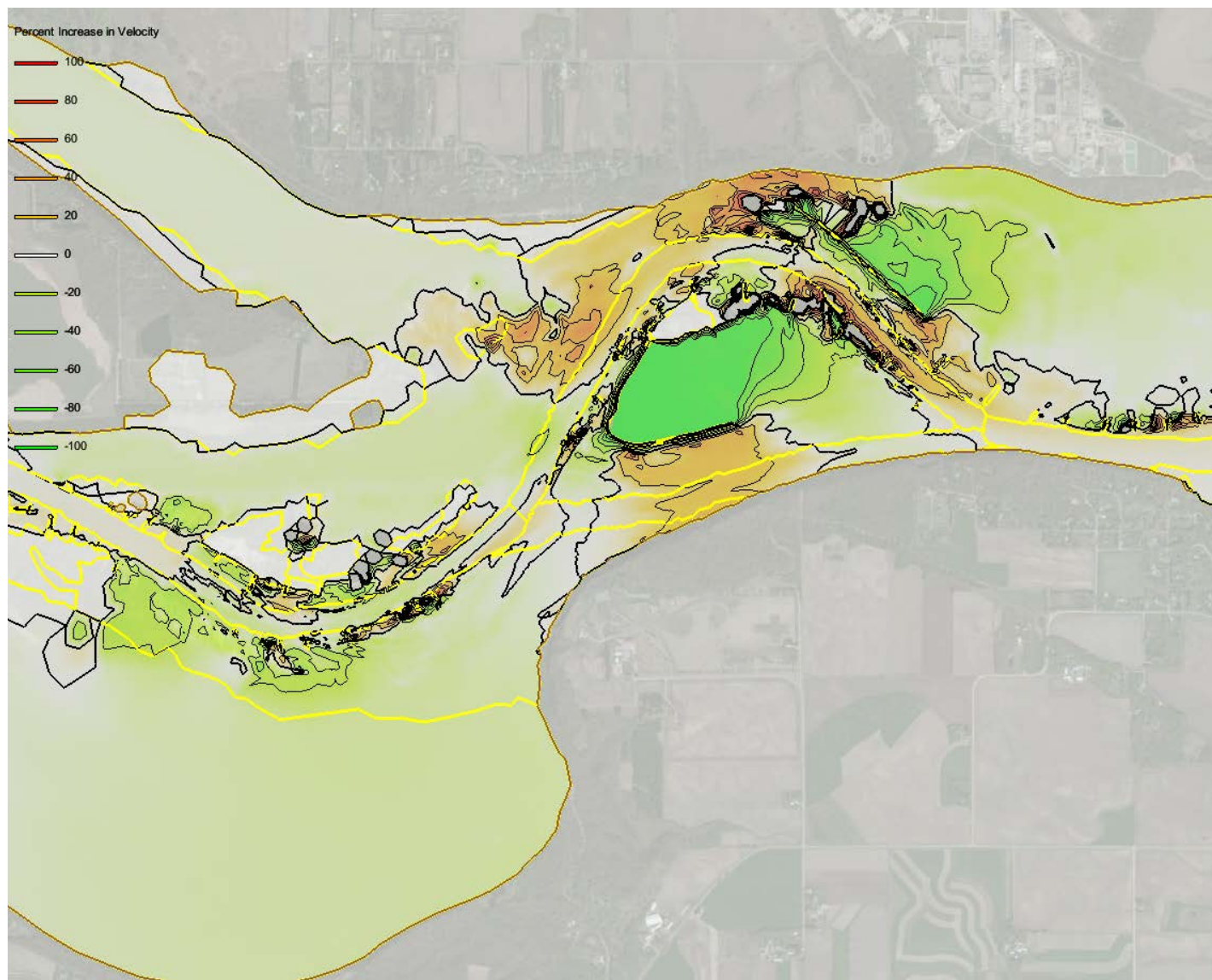
Figure 21 - Percent Increase in Channel Velocity (20,560 cfs)
