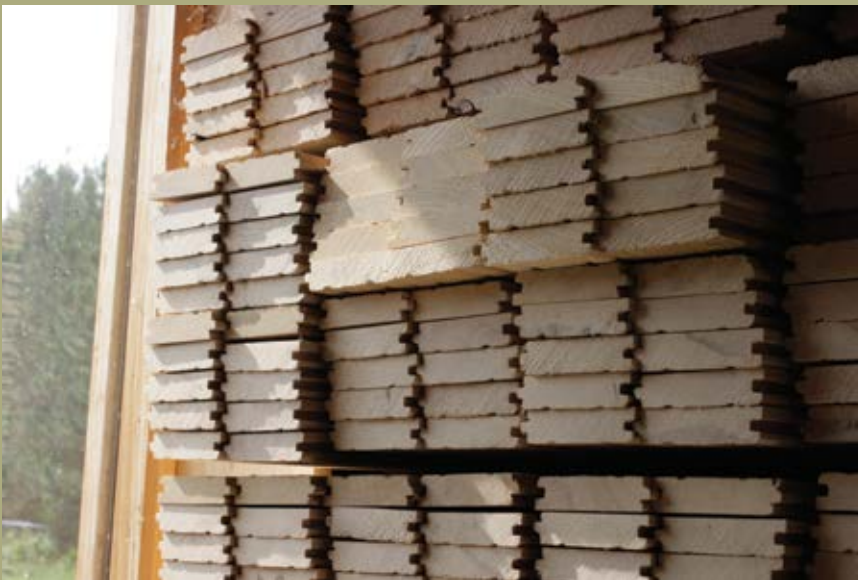
Hardwood flooring boards were dried in a solar-powered kiln.
