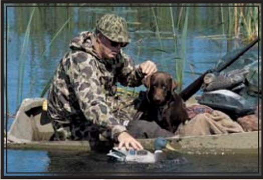
Overloading and too little freeboard is an invitation to capsizing and the most common cause of waterfowler drownings.
