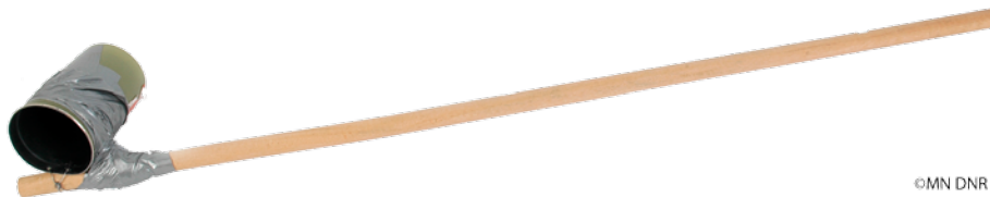
A homemade dredge, also known as the muck scooper.
