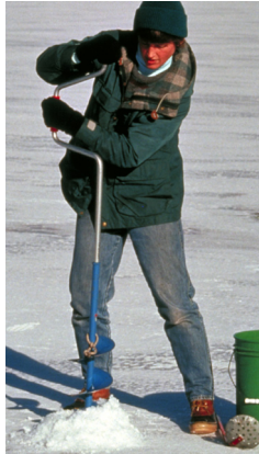
Hand augers drill holes in the ice.
