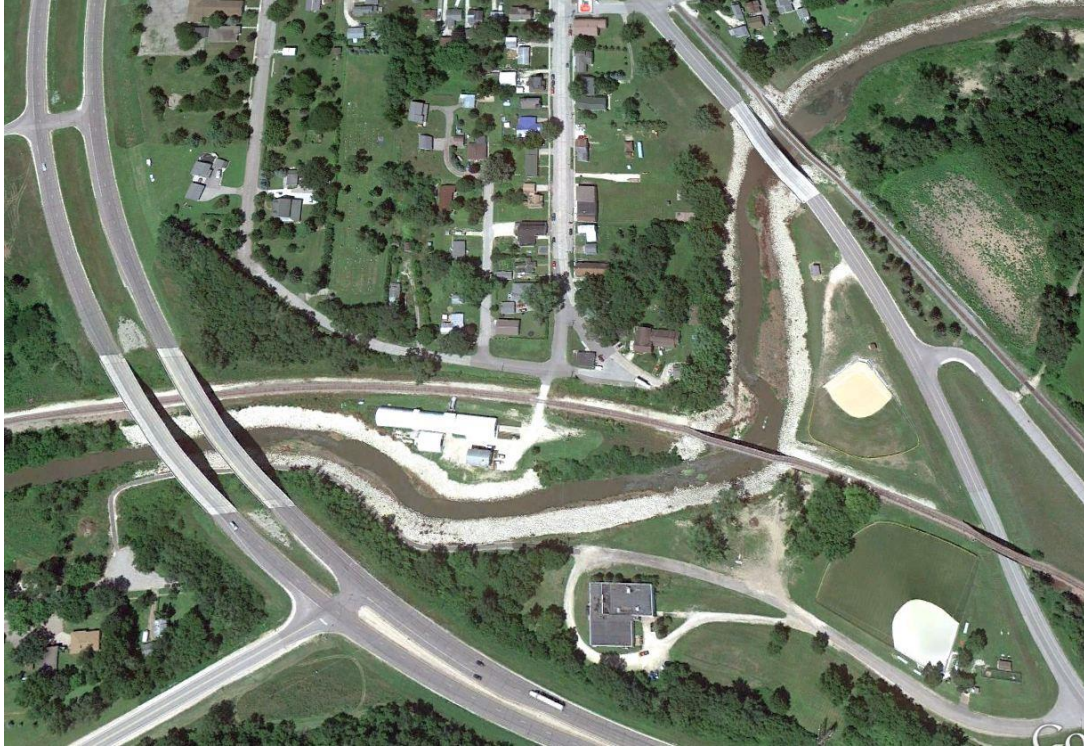
Figure 7(d): Typical Flood Flow Confinement found on the landscape. Notice the riprap lined channels which lack a defined floodplain. Over widened flat channel bottom promoting deposition and a high variability of channel widths.
