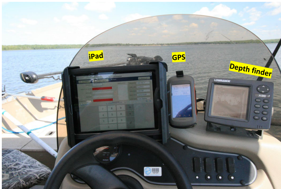
Figure A2. Using RAM mounts to secure electronic equipment to boat console
