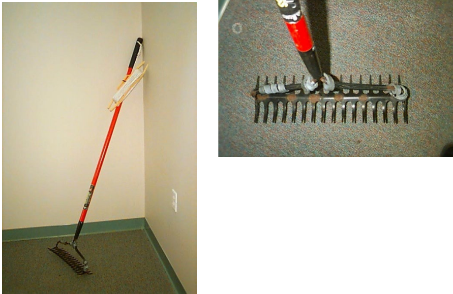
Figure A1. Double-headed, weighted garden rake for plant sampling
