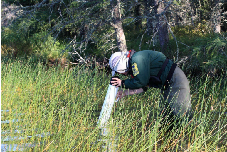
Figure A3. Commercially purchased View tube used to observe submerged vegetation
