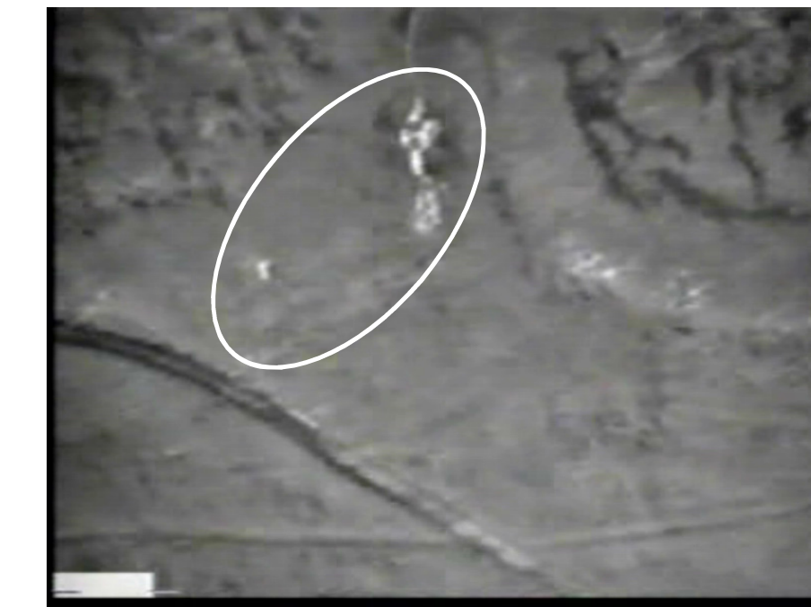
TIR image showing a groundwater intrusion area on the Knife River, January 29, 2003.
