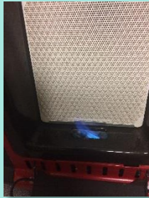
Pilot flame should be blue and sharp, indicating the pilot thermal couple is clean and operating properly. Click here to link to a You Tube video on maintenance.
