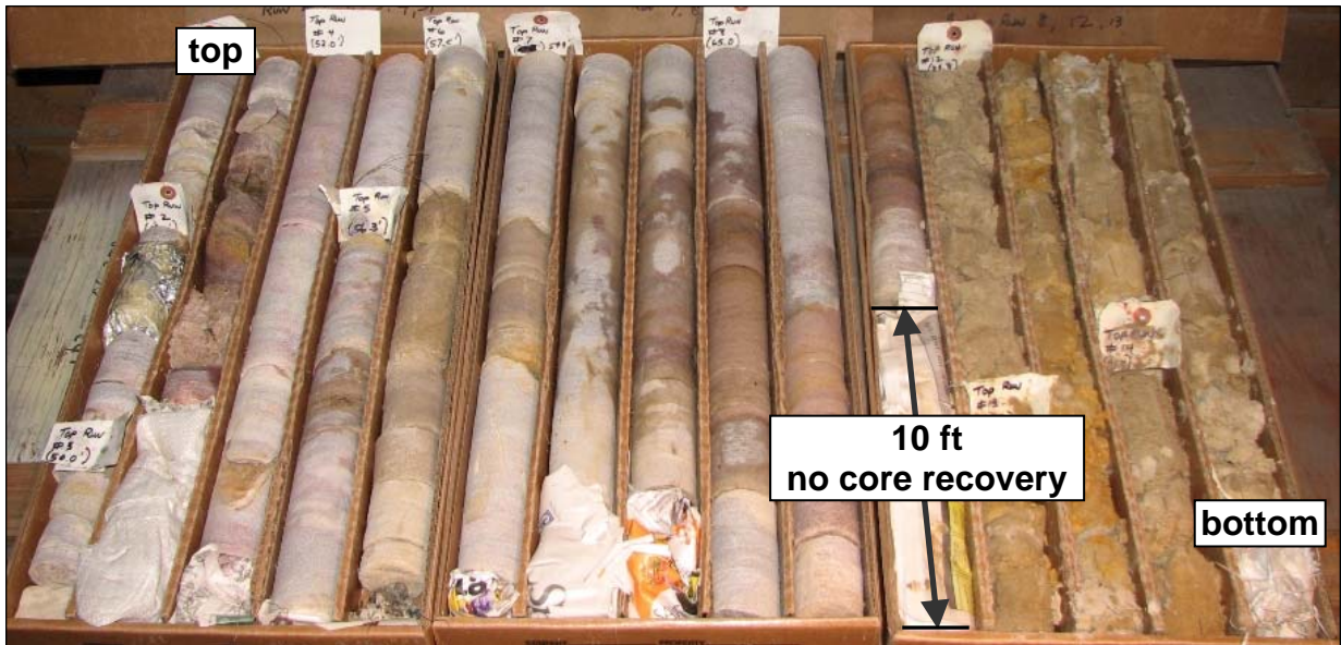
Figure 4.2 Core samples from 08-4M show a stark change in texture. Hard, well-cemented purple sandstone (left, middle) dominated at the top of the formation and transitioned to crushed, uncemented sandstone (right) below about El. 820. The transition is marked by roughly 10 ft of unrecovered core.
