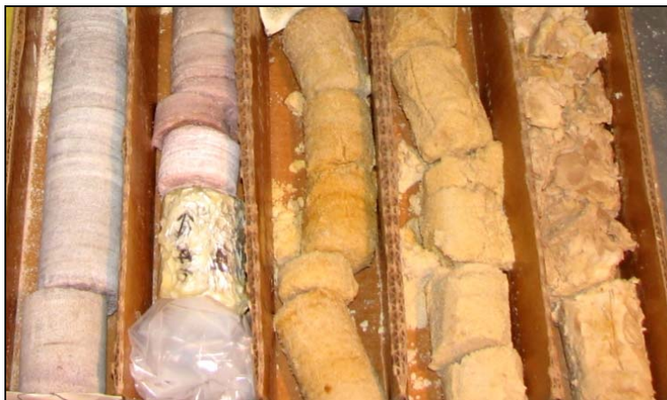
Figure 4.1 A box of rock cores from hole 08-2M showing typical variation of the Jordan Sandstone at the Rapidan Dam. Core samples ranged from hard, well-cemented, purple (left) to medium-hard with medium to poor cementation (middle) to crushed and uncemented (right).
