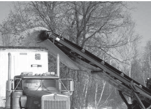
▲ New markets and policies have led to an increase in biomass utilization during forest harvest operations. Wood biomass is generally chipped on site and then loaded into trucks for transport as shown here. Photo: MFRC Staff.
