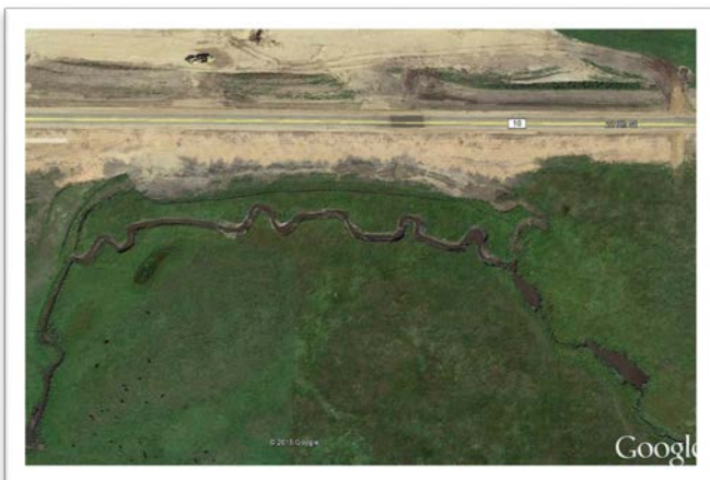
Figure 3. Re-meandered section of Flandreau Creek next to Pipestone County Road 10 in the Missouri River Basin. Traces of the old, straightened creek are visible just below the road in this Google Earth image.
