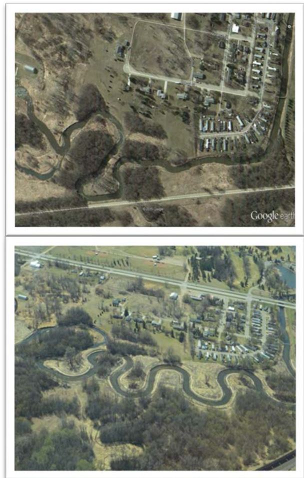
Figure 6. Buffalo River natural channel restoration at the City of Hawley, 2015: Before (top) and after (bottom).
