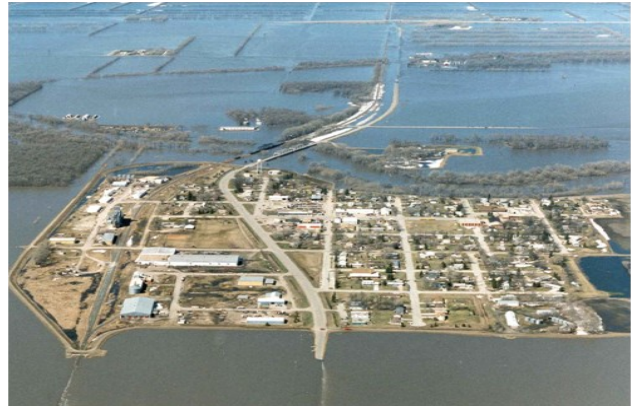
Oslo, Minnesota, largely protected by flood control structures during The Red River flood of 1997. .
