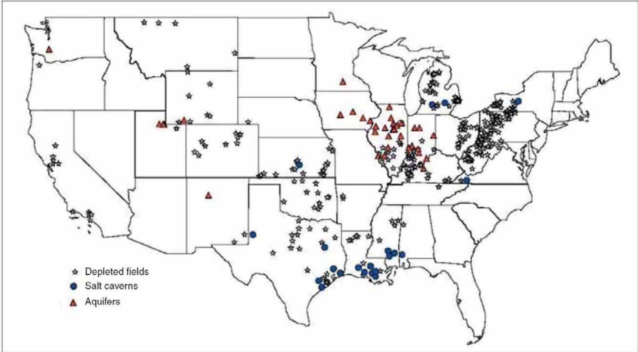
Figure 18. Underground gas storage facilities in the US (MGSC, after International Energy Agency)
