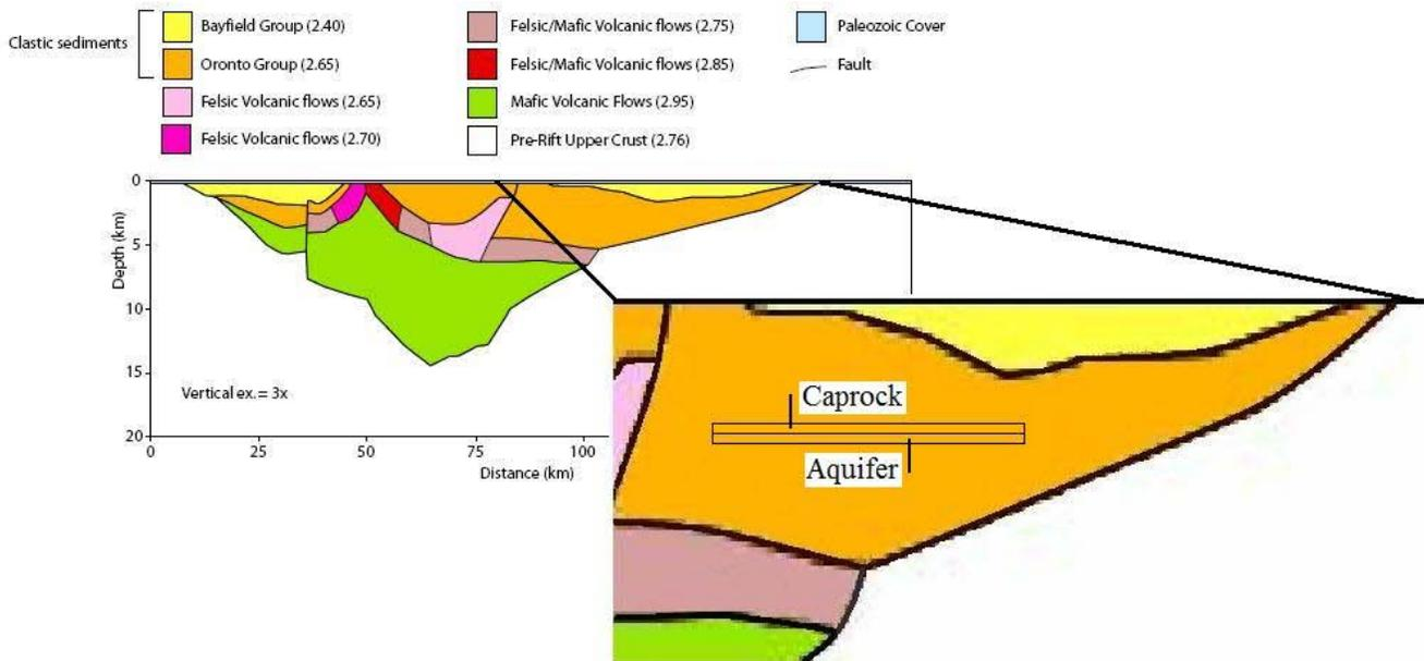
Figure 43. A conceptual model of the aquifer and caprock structure we use for the initial stage 1 and stage 2 modeling. Because of the lack of information, we assume a long, thin aquifer below a capping unit. The aquifer is within one of the sedimentary units of the Mid Continental Rift System of interest for CO<sub>2</sub> storage and is at a depth sufficient for storage.
